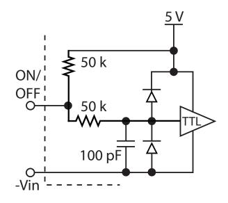
Figure B: Internal ON/OFF pin circuitry
