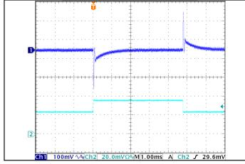
Figure 5: Output voltage response to step-change in load current (50%-75%-50% of Iout(max);  $dI/dt = 0.1A/\mu s$ . Load cap:  $15\mu F$  tantalum cap and  $1\mu F$  ceramic cap. Ch 1: Vout(100mV/div), Ch 2: Iout(20.0mA/div). Time scale(1.00ms/div).
