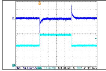
Figure 5: Output voltage response to step-change in load current (50%-75%-50% of Iout(max);  $dI/dt = 0.1A/\mu s$ . Load cap:  $15\mu F$  tantalum cap and  $1\mu F$  ceramic cap. Ch 1: Vout(50.0mV/div), Ch 2: Iout(10.0mA/div). Time scale(1.00ms/div).
