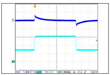
Figure 6: Output voltage response to step-change in input voltage (1000 V/ms). Load cap: 1  $\mu$ F ceramic and 15  $\mu$ F tantalum capacitors. Ch 1: Vout(1.00V/div), Ch 2: Vin(50.0V/div).Time scale(1.00ms/div).
