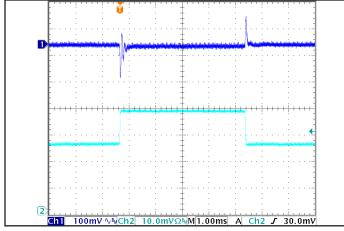
Figure 5: Output voltage response to step-change in load current (50%-75%-50% of lout(max);  $dI/dt = 0.1 A/\mu s$ ). Load cap:  $1 \mu F$  ceramic and  $15 \mu F$  tantalum capacitors. Ch 1: Vout(100mV/div), Ch 2: lout(10.0mA/div).Time scale(1.00ms/ div).
