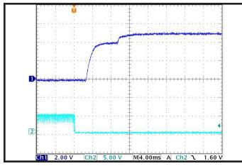
Common Figure 1: Typical startup waveform on Ch 1 (2.00V/div). Input voltage pre-applied, ON/OFF Pin on Ch 2 (5.00V/div). Time scale (4.00ms/div).
