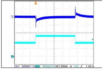
Figure 5: Output voltage response to step-change in load current (50%-75%-50% of lout(max);  $dI/dt = 0.1 A/\mu s$ ). Load cap:  $1 \mu F$  ceramic and  $15 \mu F$  tantalum capacitors. Ch 1: Vout(200mV/div), Ch 2: lout(500mA/div).Time scale(1.00ms/ div).
