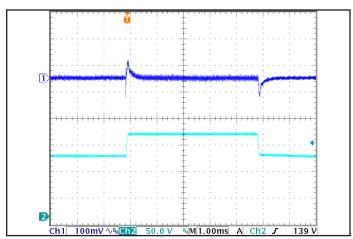
Figure 6: Output voltage response to step-change in input voltage (600 V/ms), at Max. load current. Load cap: 1µF ceramic cap.Ch 1: Vout(100mV/div), Ch 2: Vin (50.0V/div).Time scale(1.00ms/div).
