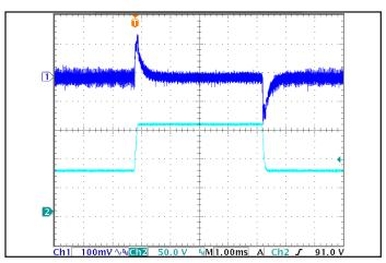
Figure 6: Output voltage response to step-change in input voltage (715V/ms), at Max. load current.Load cap:  $15\mu$ F tantalum cap and  $1\mu$ F ceramic cap.Ch 1: Vout(100mV/div), Ch 2: Vin(50.0V/div). Time scale(1.00ms/div).
