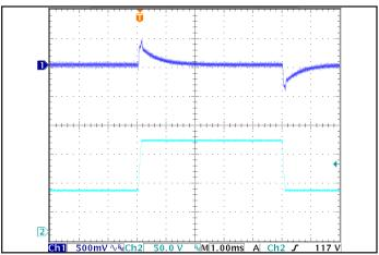
Figure 6: Output voltage response to step-change in input voltage (650V/ms), at Max. load current.Load cap:  $15\mu$ F tantalum cap and  $1\mu$ F ceramic cap.Ch 1: Vout(500mV/div), Ch 2: Vin(50.0V/div).Time scale(1.00ms/div).
